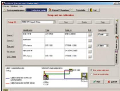
JOFRACAL calibration software may also be used for manual calibrations, as it can be set up to accept manual entry of calibration data together with other liquid baths, ice points or dry-block heat sources.
